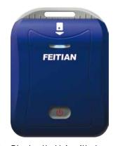
The bR301 supports Bluetooth V.4 with low energy mode and AES data encryption. The battery has a run time of 8-10 hours and is user replaceable.
